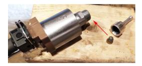
In addition to in-line fuel filters, some fuel pumps may also have a fuel screen on the inlet side of the pump. These do not normally need to be replaced but if the heater is having difficulty starting or has excessive smoking, it would be a good idea to inspect and or replace this.
